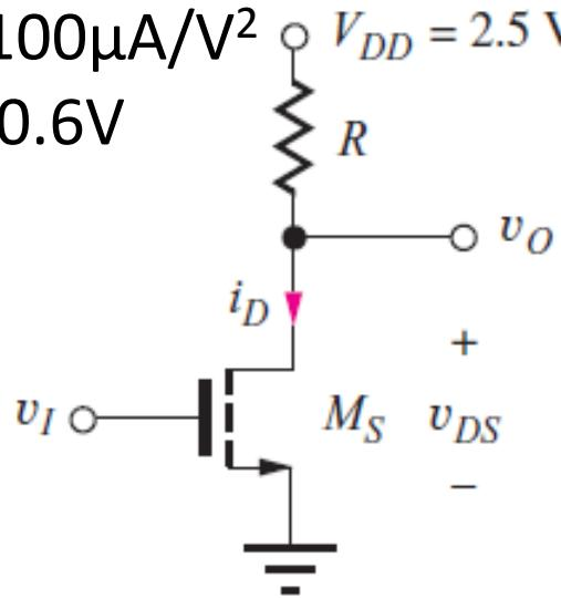
$$v_I = v_{GS}, v_O = v_{DS}$$
