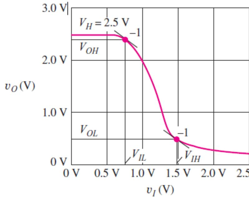
A long chain of such inverters can tolerate noise and process variations around 0.25 V in the low-input state and 0.96 V in the high state.
